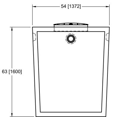
1: 4" Inlet rubber 2: 24" Diameter polylok riser
